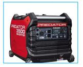
**Phoscrete Generator**: This 3500 watt inverter/generator produces more power, with a clean power curve and low fuel consumption. 212cc air-cooled OHV gas engine. Run time: 11 hours (a) 25% capacity. (2) 120VAC grounded outlets, (1) 120VAC Twisotlock Outlet, (1) DC-12V Two Pin Outlet. Electric start. Parallel capable [**1,283 points**]
